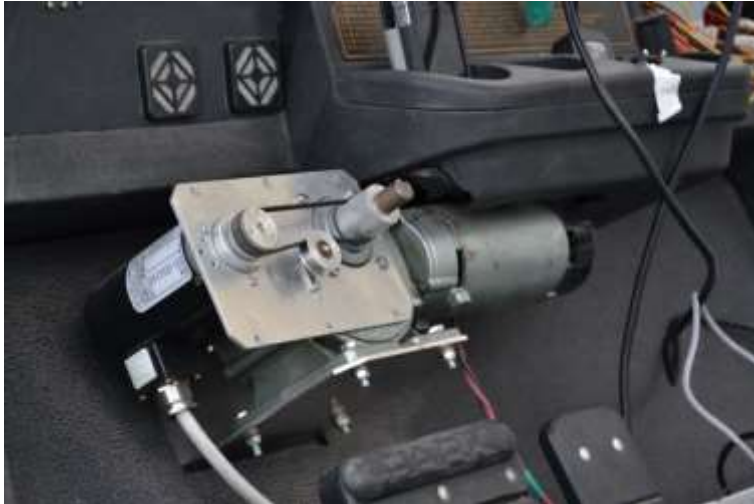
Fig. 2. iCab steering system: motor-encoder
