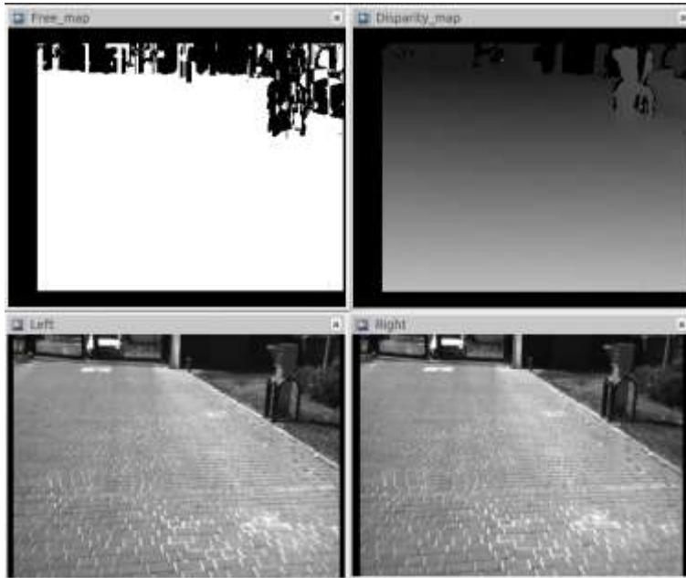
Fig. 10. Stereo images, disparity map and free map ROS-based low-level perception processes in real-time without obstacles to accomplish autonomous navigation
